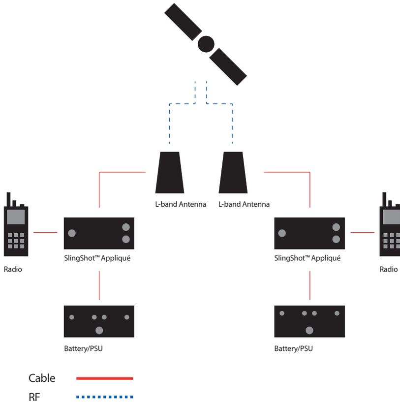
L-TAC from OneWeb Technologies leverages Inmarsat's I-4 satellite constellation and integrates Spectra's SlingShot™ to enable current UHF or coalition forces VHF radios to utilize L-band satellite frequencies to deliver BLOS communications.
